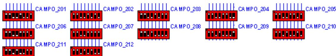
The EP095M Control Unit allows up to 60 fields, but repeats frequency every 12 so this configuration would be repeated every 12-field cycle.
